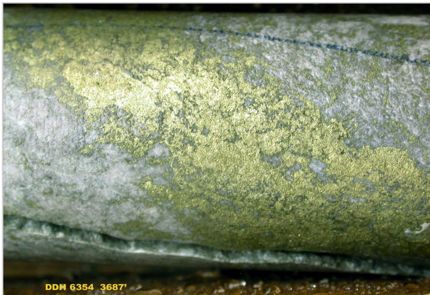
Figure 7-8: Drill Core Photograph Showing Chalcopyrite Mineralization
