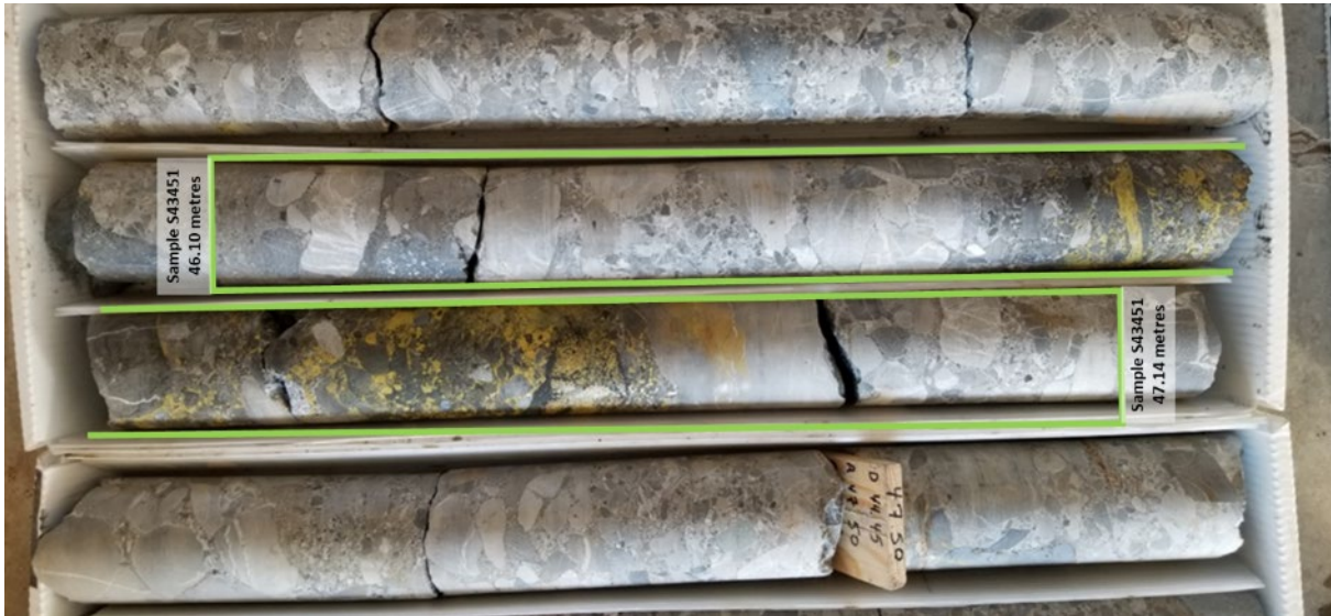
Disseminated blebs and clots of orpiment (yellow mineral) in silicified, brecciated limestone conglomerate (Pedro Drill Hole P22-02; 46.0m to 47.4m; 0.750 g Au/t; samples S43451 & S43451R)
