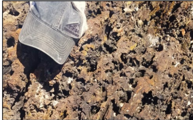
Tertiary-age silicified limestone conglomerate breccia with arsenopyrite, pyrite, realgar and orpiment mineralization located on the Centauro Gold Project. On left, surface grab sample 796074: 0.072 g Au/t.
