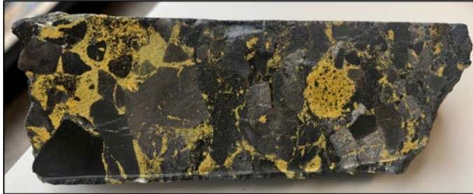
Pedro Gold Project: Quartered HQ-size drill core specimen with orpiment mineralization (yellow) replacing limey matrix in silicified, brecciated limestone conglomerate (0.750 g Au/t; averaged samples S43451 & S43451R; hole P22-02; 46.0m to 47.4m).
