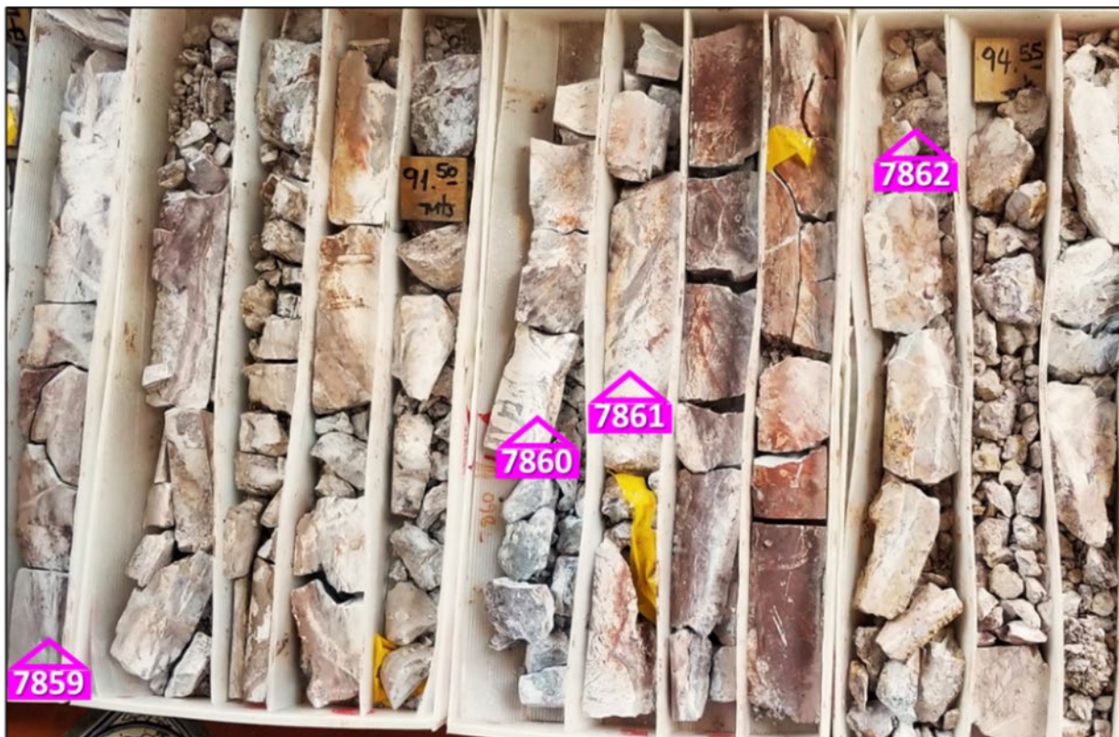
Drill core from hole CEN08-10 exhibiting intense argillic alteration (kaolinite) and averaging 232 ppb Au, 5.5 ppm Ag, 1,328 ppm As, 102 ppm Hg, 50.8 ppm Sb and 4.4 ppm Mo over a 6.7 m interval starting at 88.4 m (weighted average of samples 7859 through 7862).
