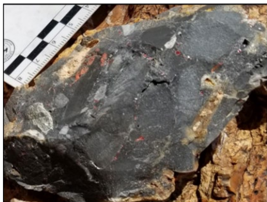
Tertiary-age silicified limestone conglomerate breccia with arsenopyrite, pyrite, realgar and orpiment mineralization located on the Centauro Gold Project. On left, surface grab sample 796074: 0.072 g Au/t.
