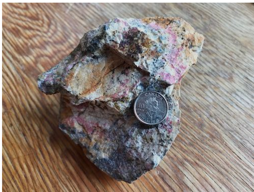
Figure 28: Cobalt bloom on surfaces of molybdenite-mineralized breccia Red Mountain molybdenite deposit
