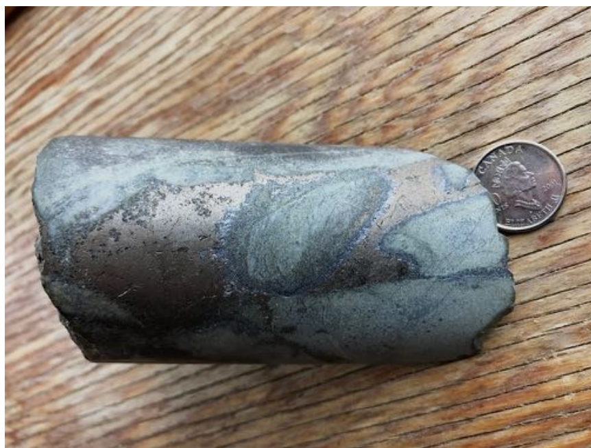
Figure 29: Epidote alteration in pyrrhotite-molybdenite mineralized breccia, Red Mountain molybdenite deposit
