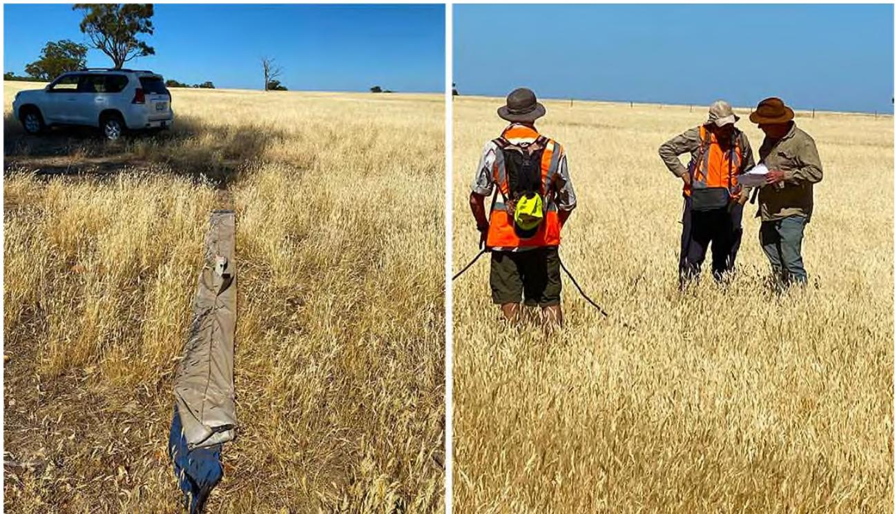
Fig. 1 – DGPR antennas being laid out before the measurement is taken (left hand photo) Denis Walsh assisting with directions with geophysicist Derek Reeves (right hand photo).
