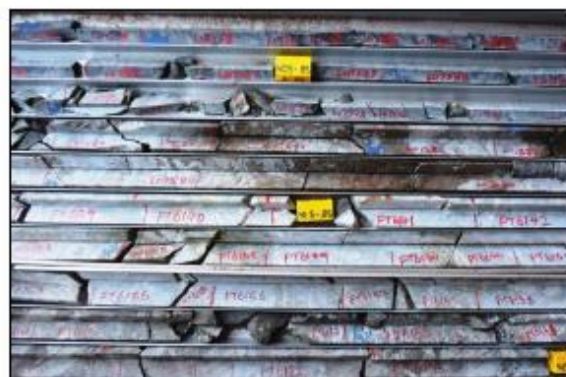
Massive sulphide zone towards the base of drill hole Z017.
