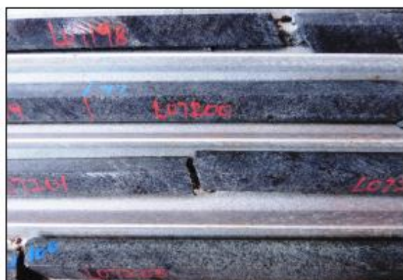
Disseminated Ni-Cu sulphides in serpentinized dunite, drill hole Z017 Lower Zone.
