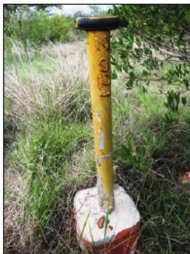
Collar stand pipe for drill hole Z021.
