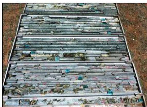
Drill hole Z01 showing faulted contact between serpentinized dunite and Platreef-style feldspathic pyroxenite.
