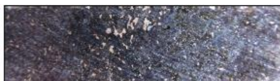
Blebby and disseminated Ni-Cu sulphides in serpentinized dunite, drill hole Z017 Lower Zone.
