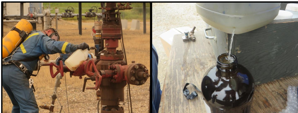
Figure 11: Sample collection at wellhead. Left: Maxxam employee sampling from access port into 4 L plastic container. Right: Decanting brine sample from bottom of 4 L container.
