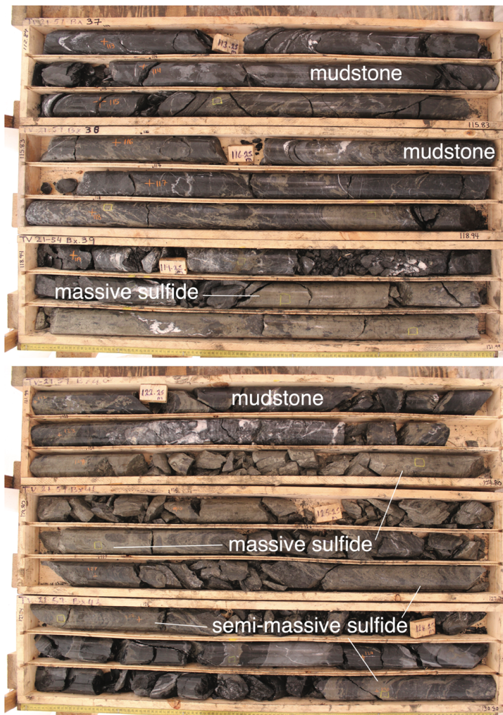
TV Lower Zone massive sulfide mineralization intercepted by TV21-57.
