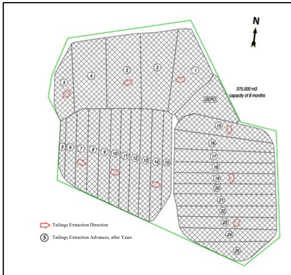
Figure 1-3: Conceptual Extraction Sequence for the CMP Tailings
