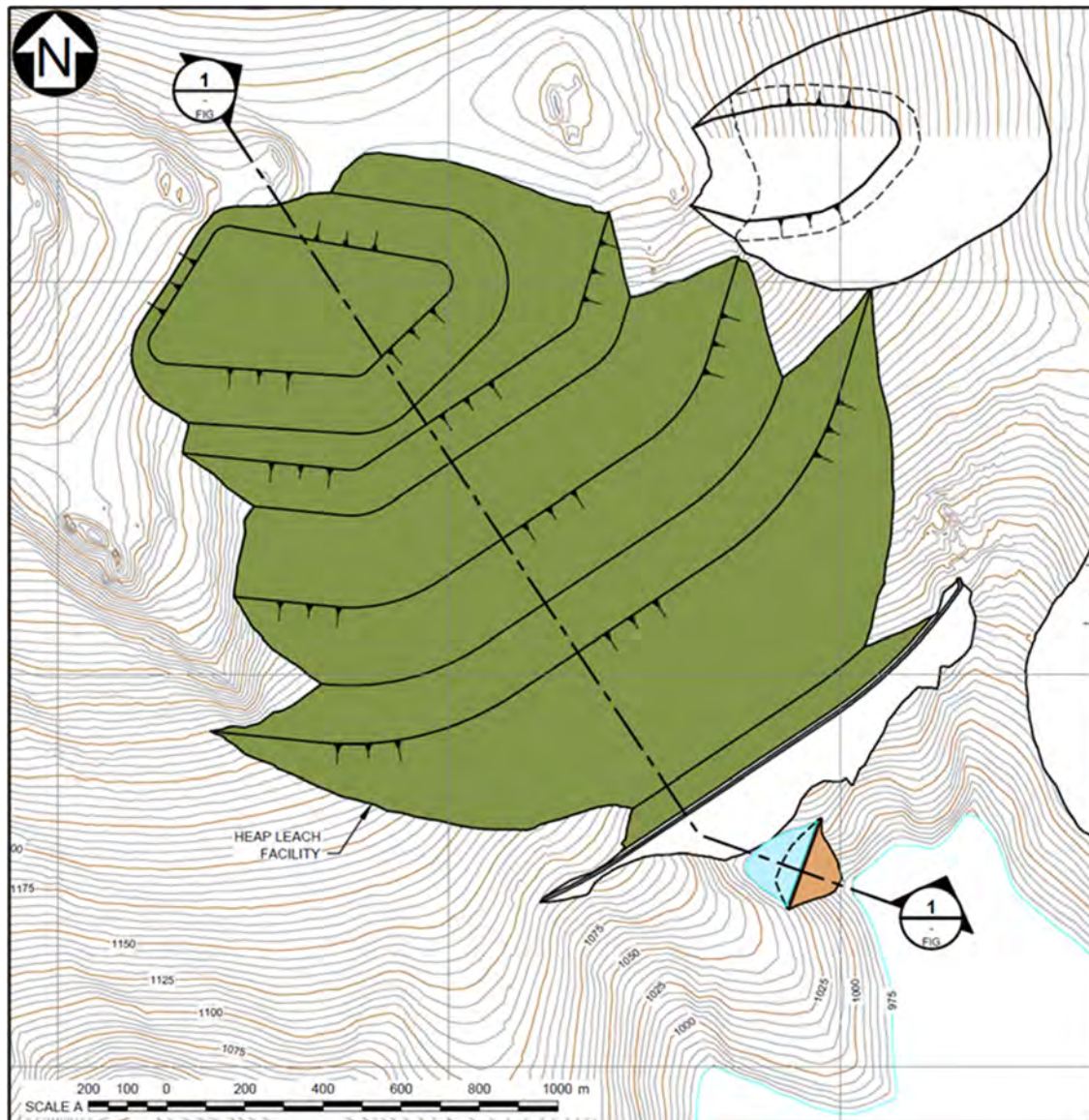
Figure 18-8: Heap Leach Facility General Arrangement (KP, 2021)
