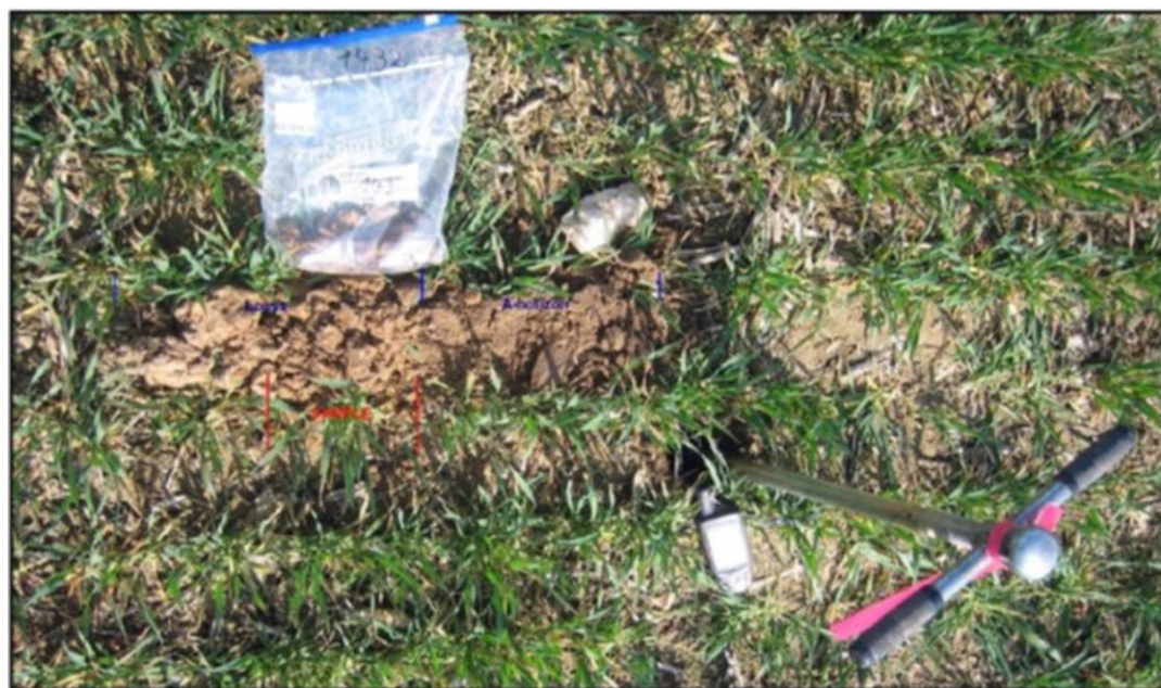
Figure 10-1 Soil sampling showing the sampled interval representing the subsoil (B horizon)
