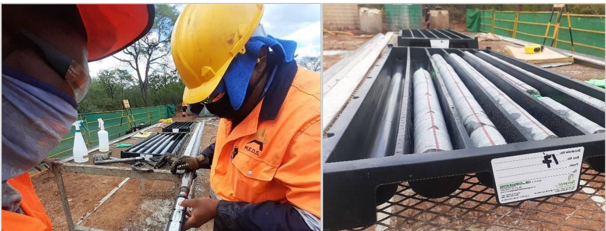
Figure 10-2: Drill core orientation performed by Mindea.
