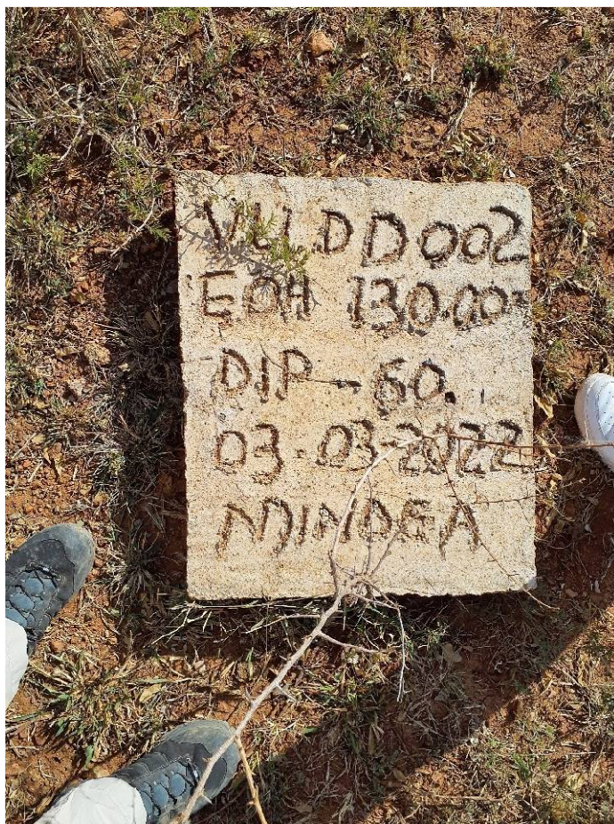
Figure 12-3 Monument for completed drill hole. Casing was removed when the hole was completed to reduce drill costs.
