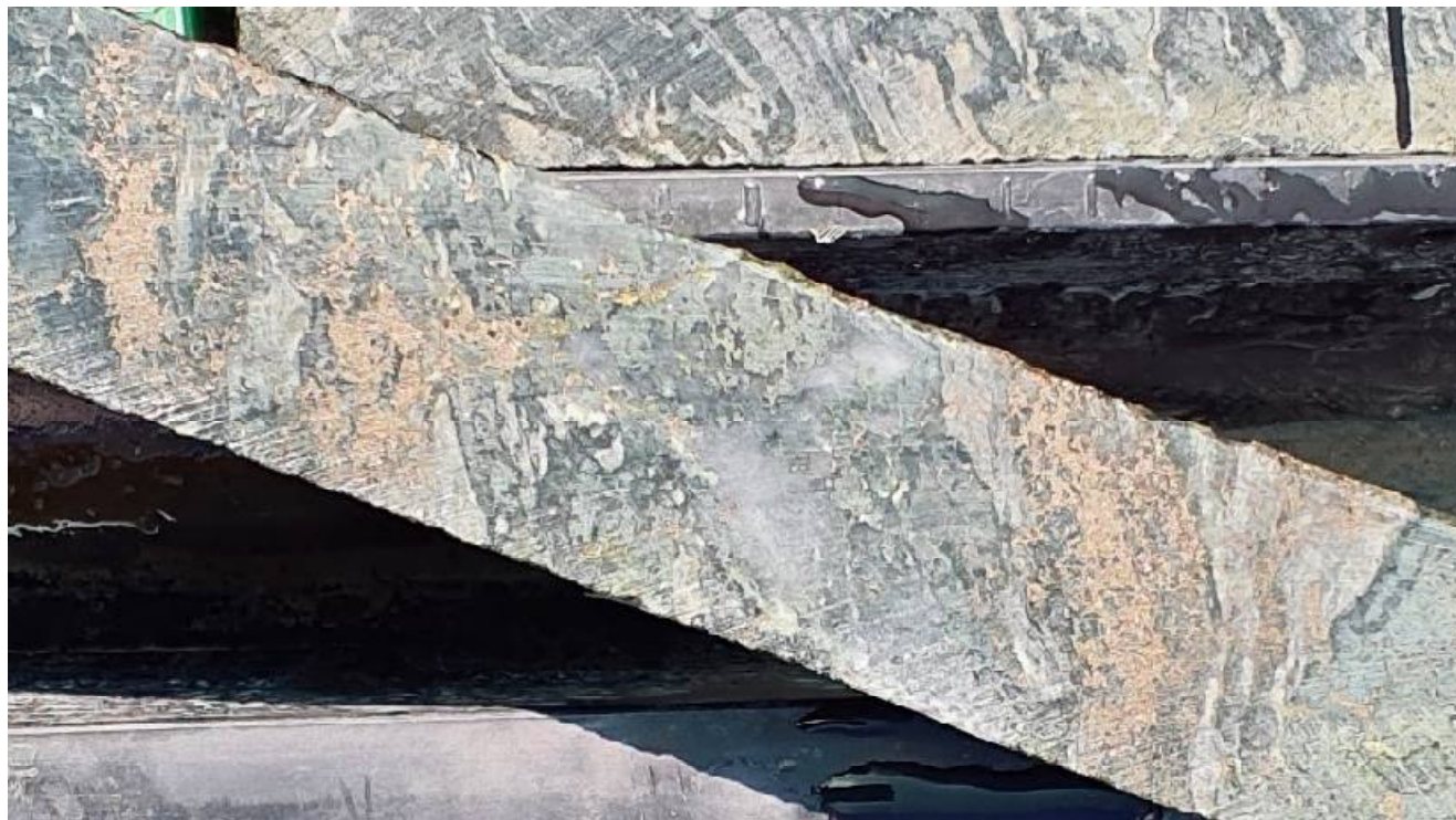
Figure 7-4: Sulphides in VUDD012 just above 91m down hole (2.13g/t Au from 90.00m to 91.00m).
