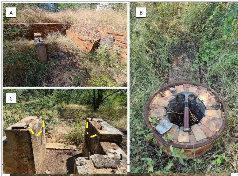
Figure 9-1: Remnants of the old processing plant. (A) Primary crushing and conveyor ruins feeding the mill, (B) small smelter with outlet at the bottom and (C) ruins with cylindrical grind marks of a small mill (Photos provided by Scholtz, 2022)
