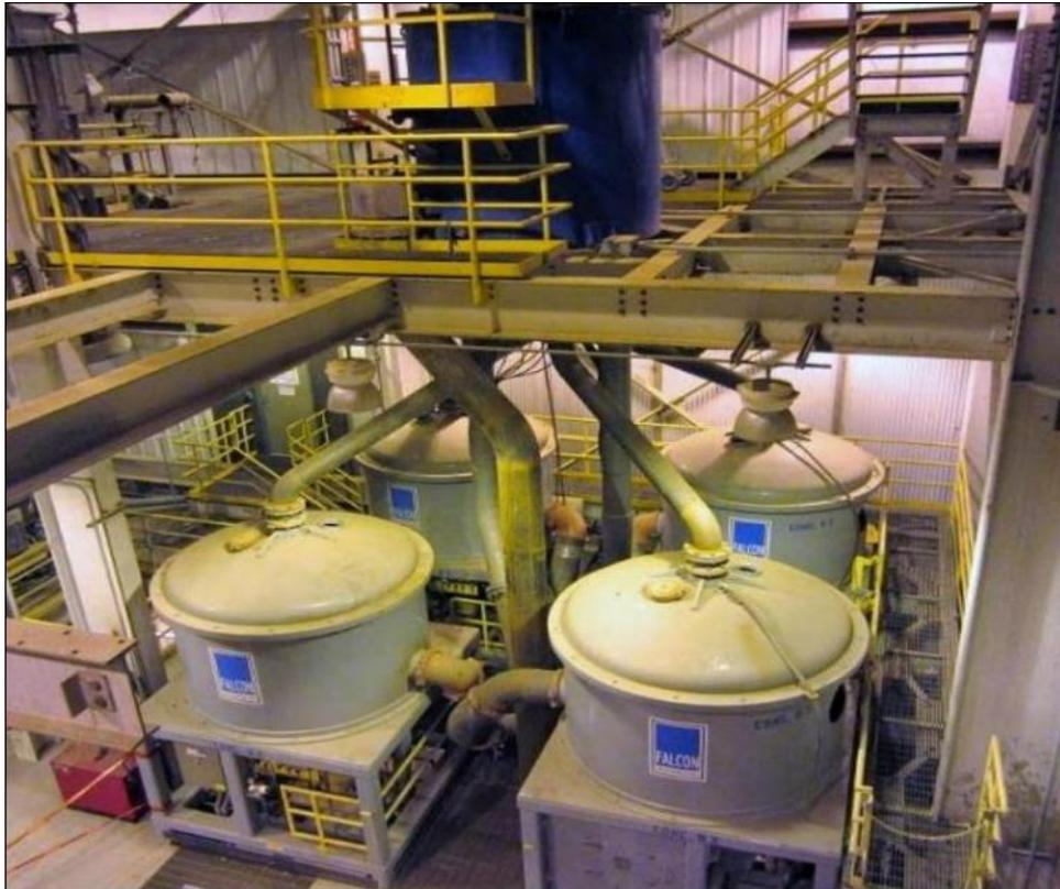
Figure 17-6 Four Falcon Gravity Concentrators
