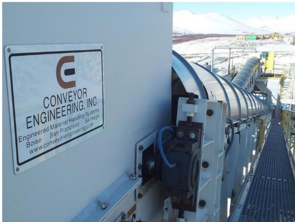
**Figure 17-4** Recirculating conveyor in Tertiary Crushing Stage
