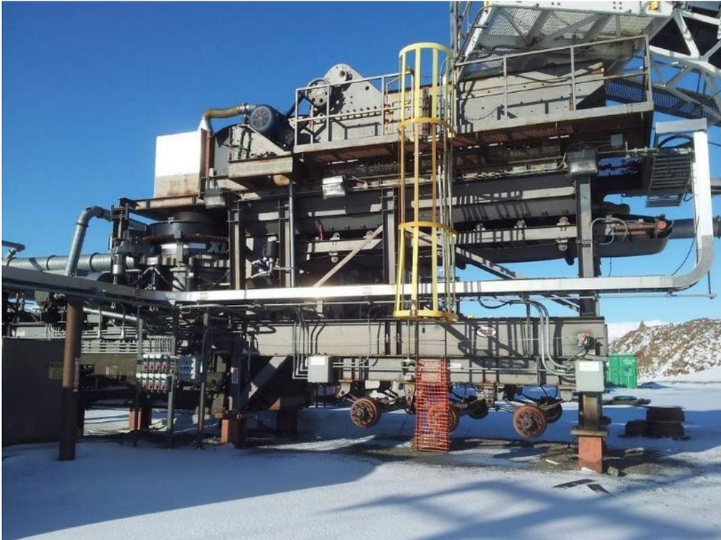
**Figure 17-3** Secondary Crusher and Vibrating Screen
