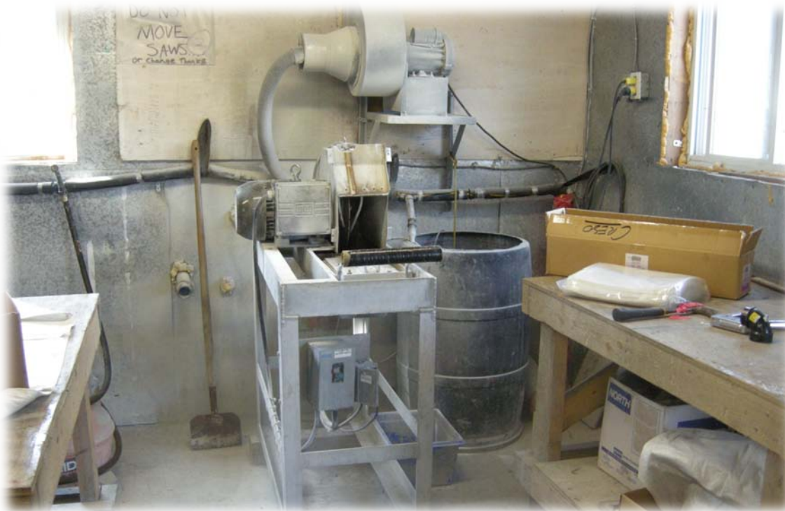
Plate 10-4: Tyranite core cutting facility.
