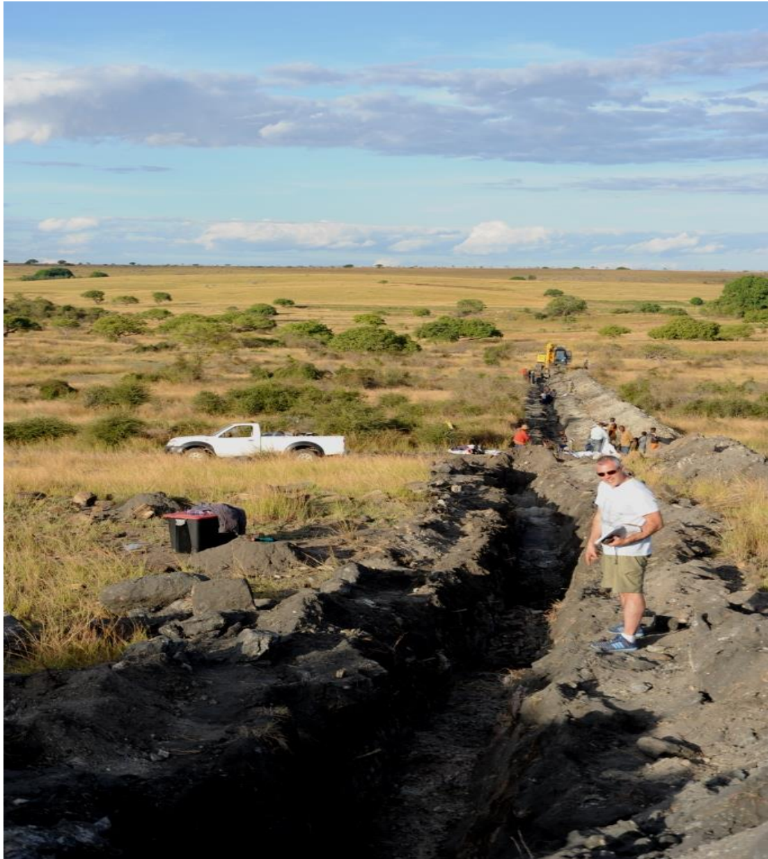
FIGURE 16: TRENCHING FOR THE BULK SAMPLE ON MOLO, MAY 2013
