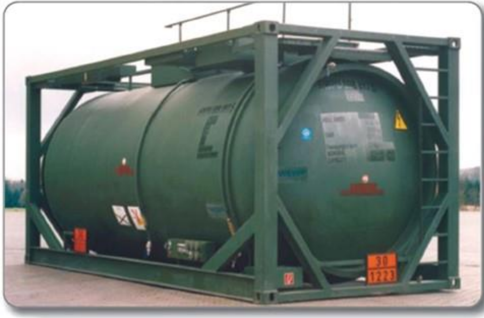
FIGURE 81: TYPICAL LAYOUT OF CONTAINERIZED FUEL STORAGE TANK
