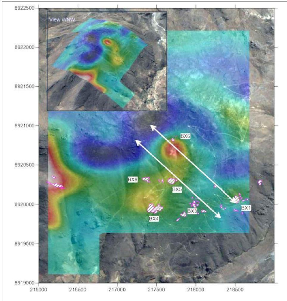
Between June 28 and July 9, 2017 SouthernRock Geophysics carried out Fixed-loop Transient EM (“FL-TEM”) & Controlled (“CSAMT”) and Natural Source Audio-frequency Magneto-Telluric surveys at Soledad (Barrett, 2017). Survey parameters followed those recommended by AGI, but with expanded coverage, such that the CSAMT survey was done along eight 135° -oriented survey lines, variably spaced at 100 or 150m.
