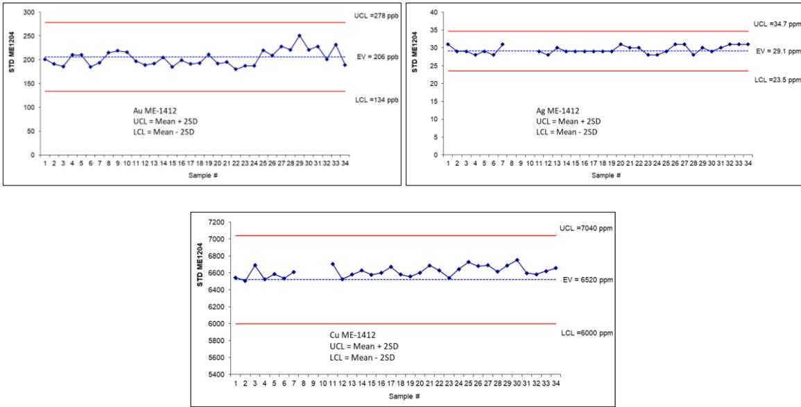
ME1412 is a polymetallic standard. No failures noted.
