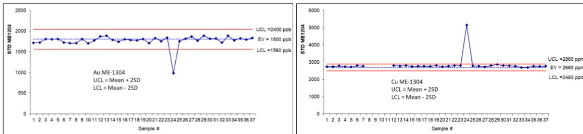
ME1304 is a polymetallic standard. There is a failure in points 24/25. This shows in silver as well.
