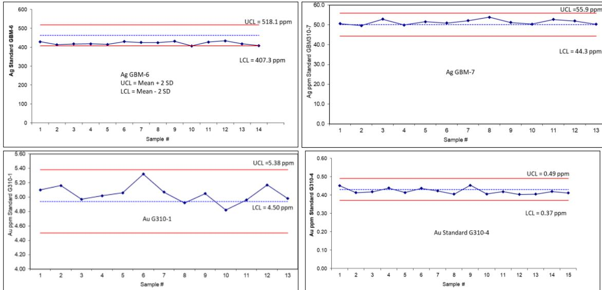
GBM-6 is a high grade silver standard. No analyses exceed the certified assay and no results exceed 2SD.
