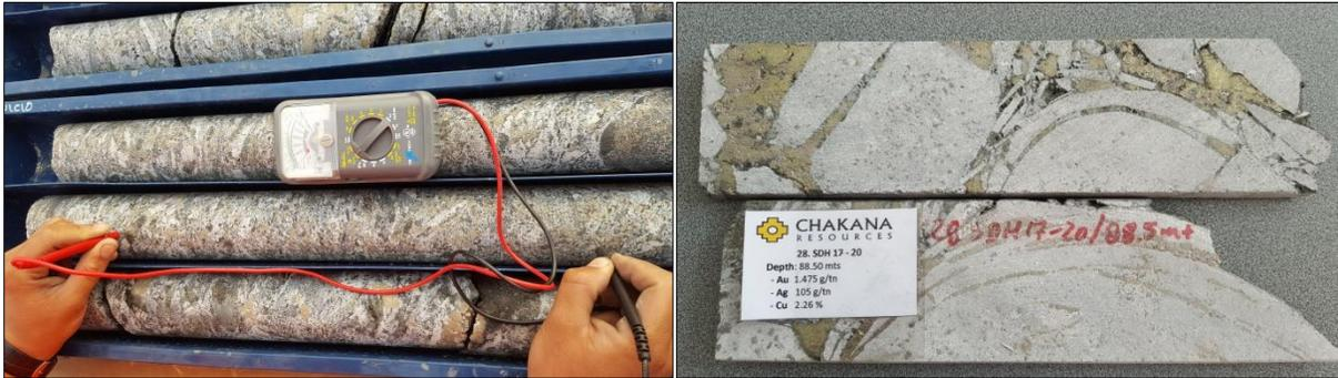
Upper left shingle breccia with strong conductivity along 50 cm length of core. Upper right shock textures, chalcopyrite – pyrite matrix.
