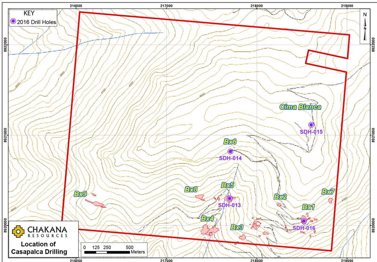
SDH-015, located in the north-east part of the project, approximately 1km to the northeast of SDH-014, was designed to test the Cima Blanca epithermal high sulphidation target, and was completed to a depth of 443m. It did not encounter significant mineralization.
