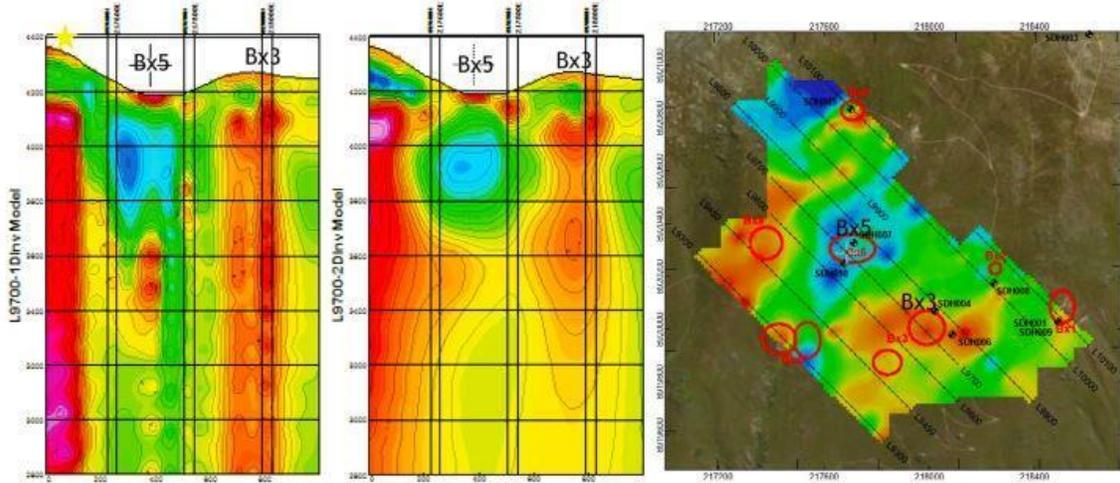
*Fig. 5.3c Soledad, 2017 CSAMT survey, Line 10100, 1D (left), & 2D (middle) inversion model resistivity sections and at 200m depth slice (right), breccia occurrences (red dash circles) and drill hole collars (black quartered symbols). Breccia 1 and 6 located on section and in plan map*
