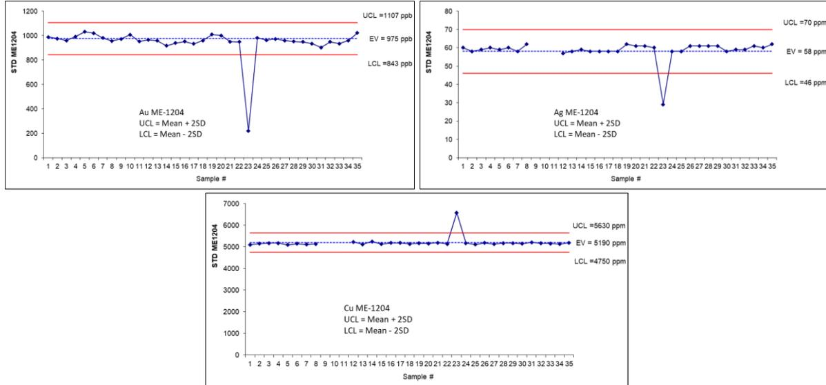
ME 1204 is a polymetallic standard. There is a through going failure in point 23, corresponding to a sample shipment from SDH-016
