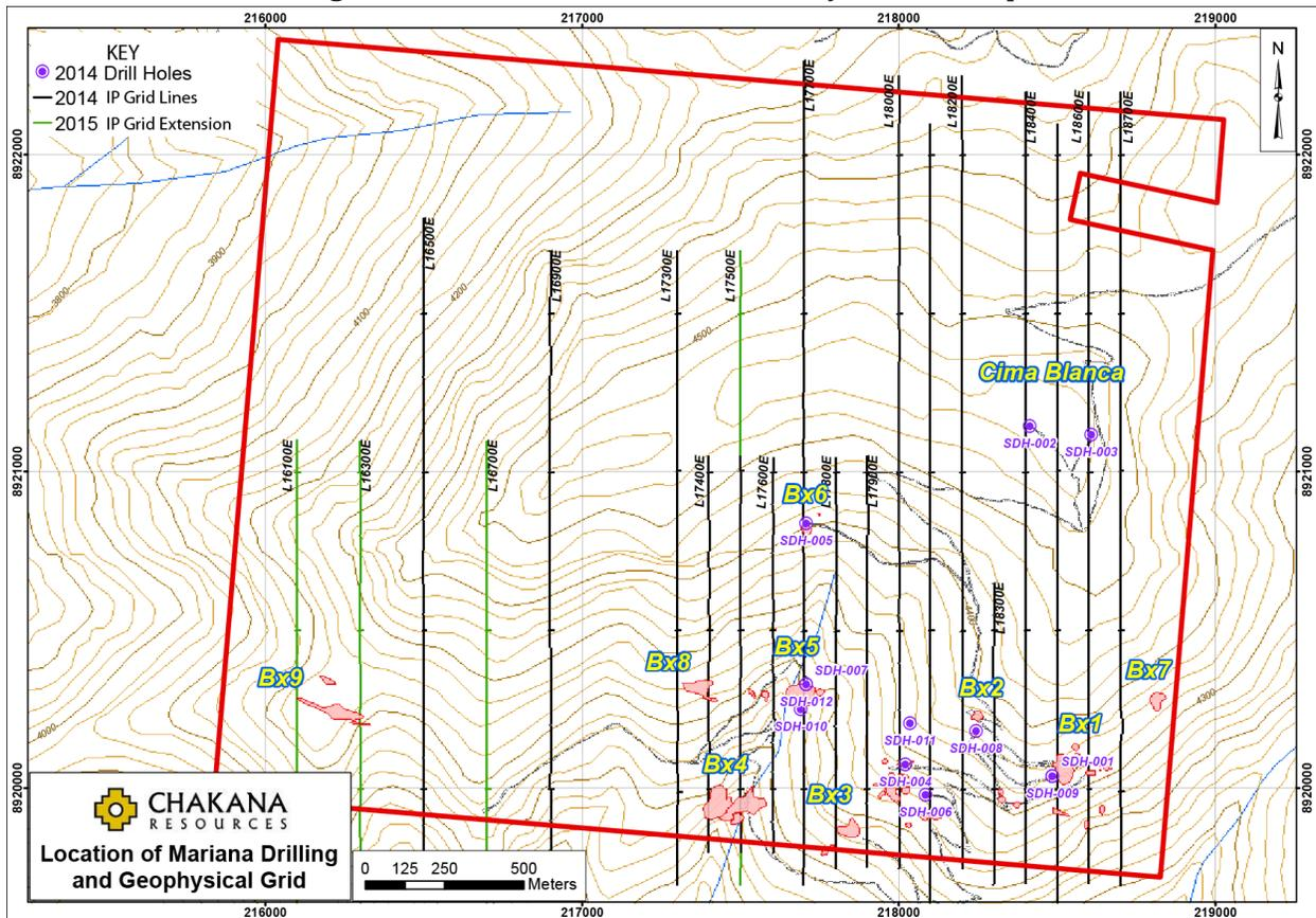
Mariana's first hole, SDH-001, located in Breccia #1, was planned as a validation hole twinning DDH-005 drilled by Rio Amarillo in 1996. The depth and grade are similar to the 1996 results, which reported 28.5m of 1.1% Cu, 5.0 g/t Au, and 28 g/t Ag.
