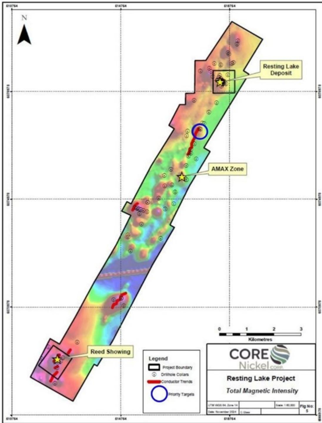
**Figure 5 - Resting Lake Project VTEM Conductors**
