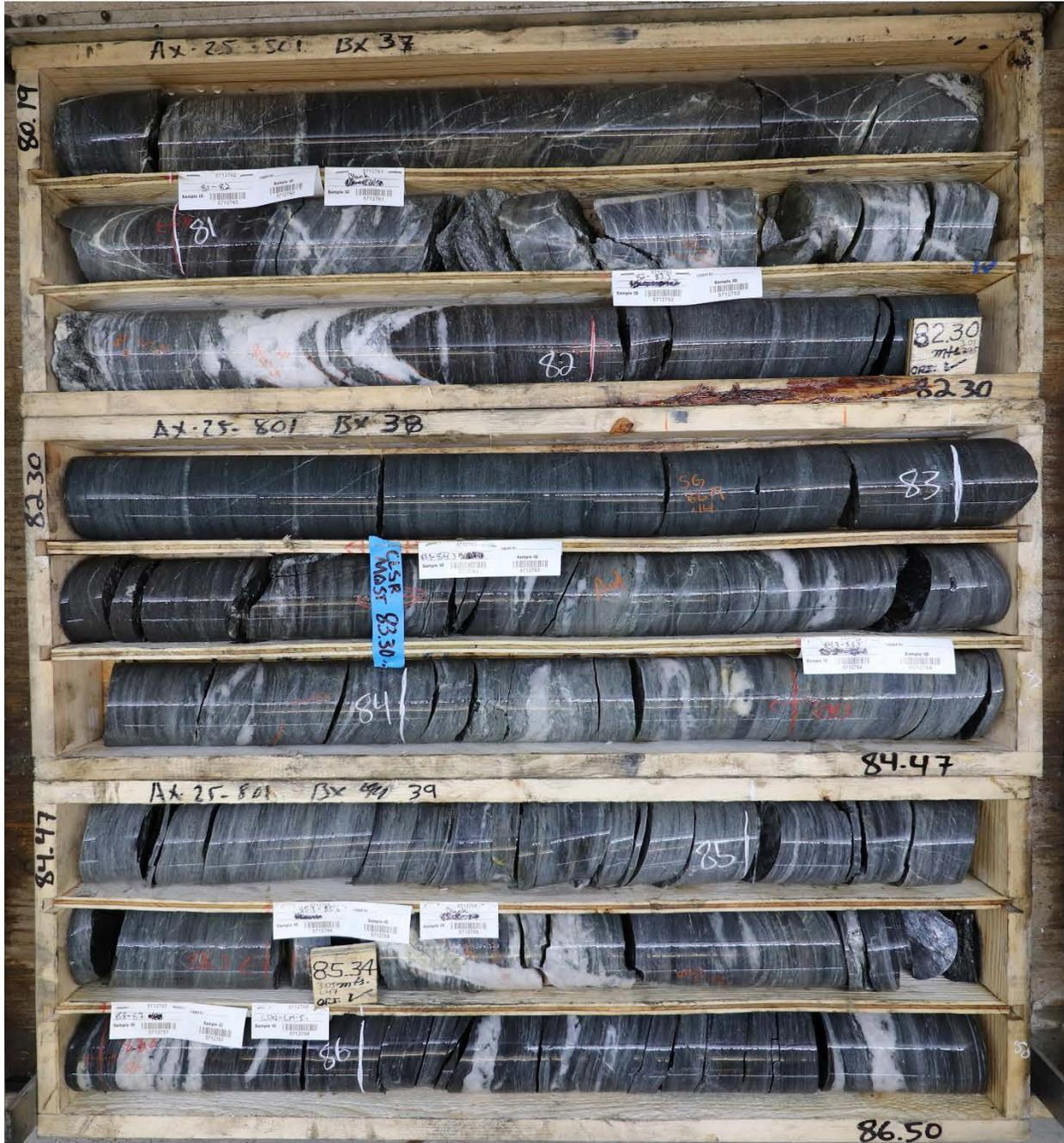
Figure 5: Diamond drill core from AX-25-801. discordant quartz veins with accessory Bi-sulphosalts, arsenopyrite, and visible gold (See Figure 2).
