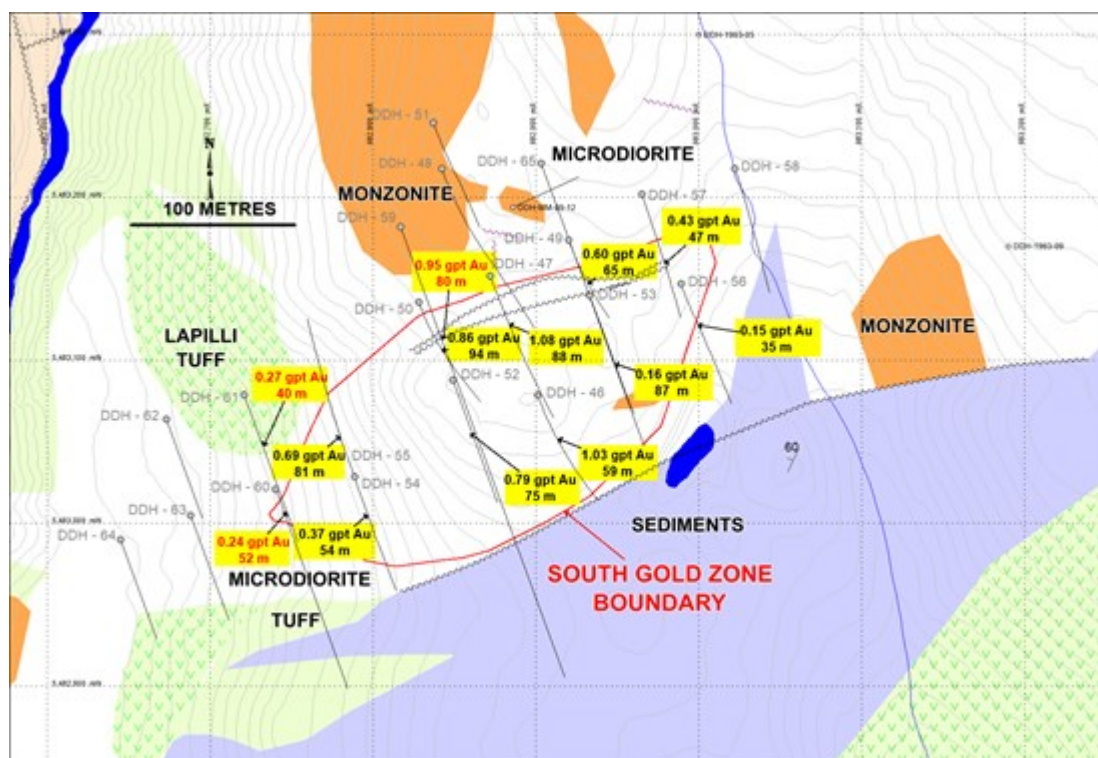
Figure 1. Recent (red) and previous (black) Au values and meterage plotted within the Southern Gold Zone Boundary on a geological plan.
