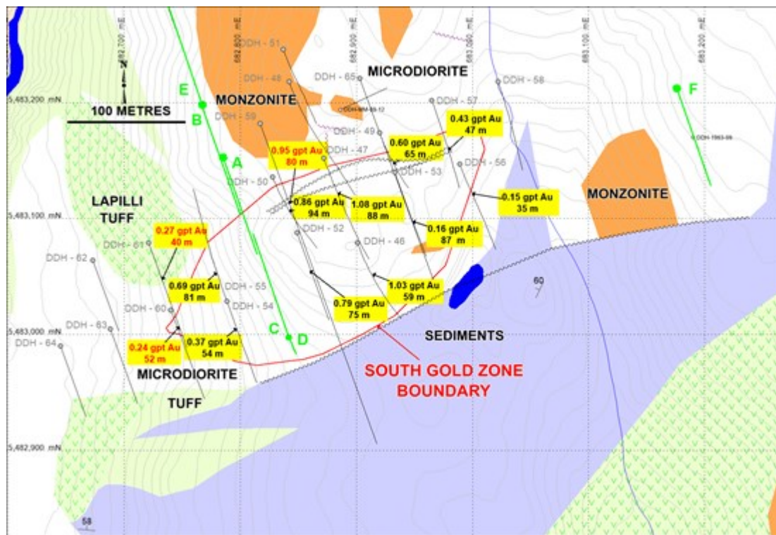
Figure 2 Proposed drill holes labelled A to F shown in bright green in the Southern Gold Zone and Au over metres values plotted on a geological map. The trace of proposed hole E will extend 2 times longer north than shown on the figure.
