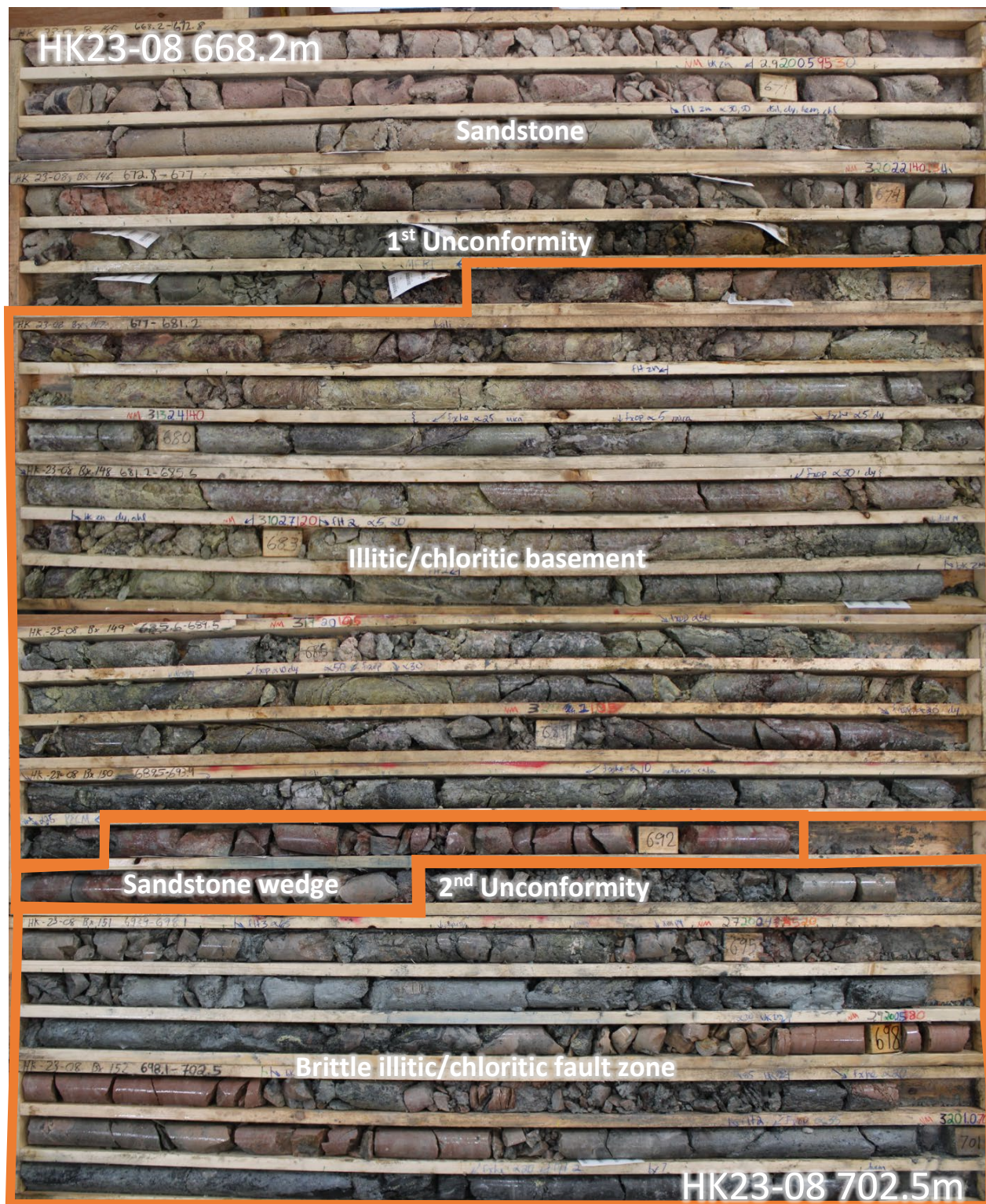
Figure 5 – Core photos from 668.2 m to 702.5 m downhole in drill hole HK23-08 illustrating strong alteration with a fault zone in the lower sandstone and upper basement. The unconformity between the sandstone and basement gneisses was intersected twice in this hole as the unconformity is structurally repeated across a fault strand within a broader altered fault zone. Refer to the cross section in Figure 4 for the location of the photographed interval and for the interpretation of fault offset of the unconformity.
