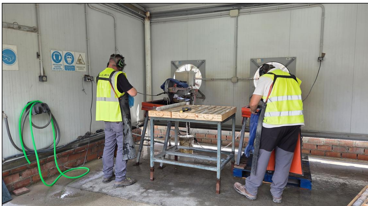
Figure 11-5 Drill Core Cutting at Pan Global's Aznalcóllar Facility
