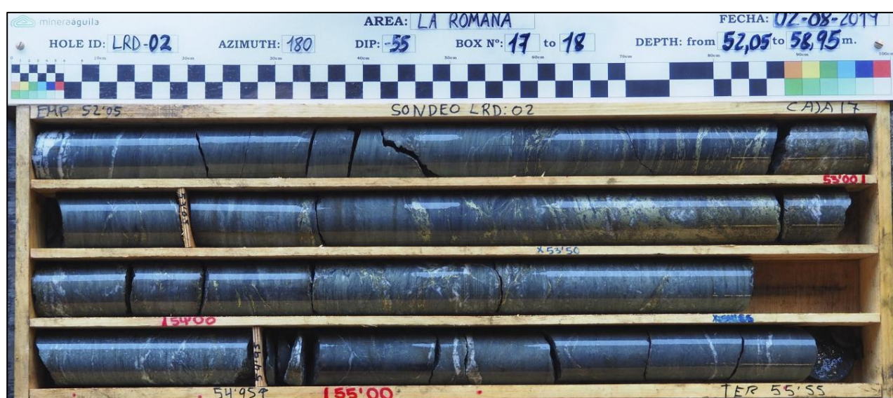
Figure 7-9 Photograph of Typical Drill Core from Diamond Drilling at La Romana
