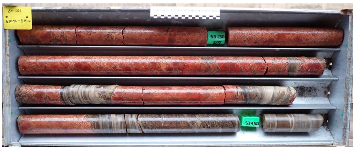
Figure 4. Potash mineralization in drill core from BA-002 Extension showing nodular red carnallite with banded bedded halite attributed to Cycle III (Dip=-90°).
