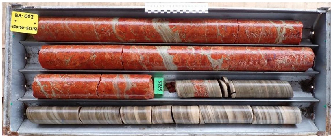
Figure 3. Potash mineralization in drill core from BA-002 Extension showing nodular red carnallite and laminated halite attributed to Cycle IV (Hole Dip=90°).
