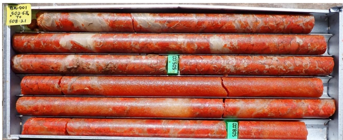
Figure 6. Red carnallite-rich core from BA-001-EXT showing interbedded nodular carnallite and halite with soft sediment deformation features at approx. 503m to 508m depth.
