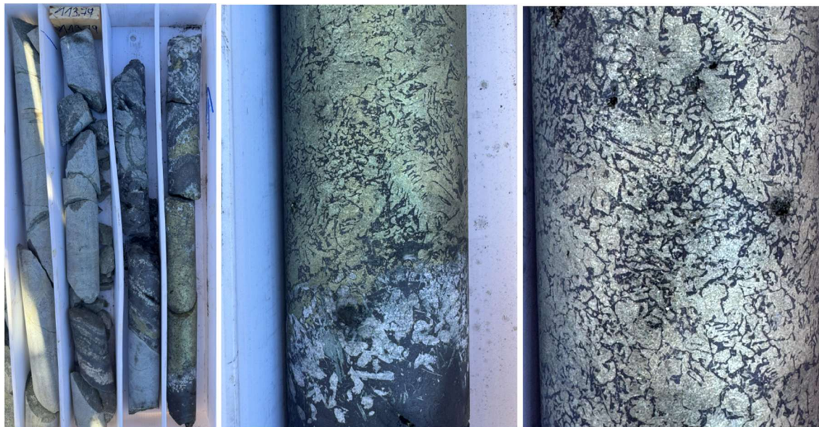
Figure 10. Drill core photographs from Hole 25SB-004 (Sample 648082) showing massive chalcopyrite replacing apatite and actinolite in a magnetite matrix
