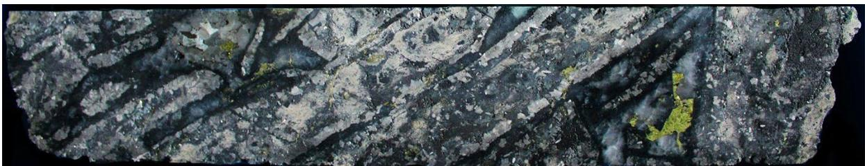
**Figure 10 – Typical high-grade copper mineralisation in drill hole CHT-DDH-041:** Shingle quartz-tourmaline breccia with clasts being replaced by arsenopyrite. Strong arsenopyrite-chalcopyrite-pyrite mineralisation. From a sample interval (227.7 to 228.43 m) that returned 0.97 g/t Au, 40 g/t Ag and 1.86 % Cu. Photograph is of a selected interval and is not necessarily representative of mineralisation hosted throughout the property.
