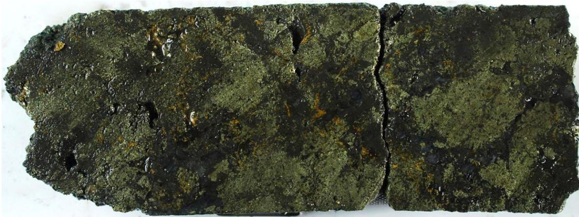
**Figure 7– Typical high-grade copper-silver mineralization in drill hole CHT-DDH-041:** Quartz-tourmaline-arsenopyrite-chalcopyrite-pyrite breccia. From a sample interval (167.06 to 167.9m) that returned 14.8 % Cu, 373 g/t Ag and 1.04 g/t Au. Photograph is of a selected interval and is not necessarily representative of mineralisation hosted throughout the property.
