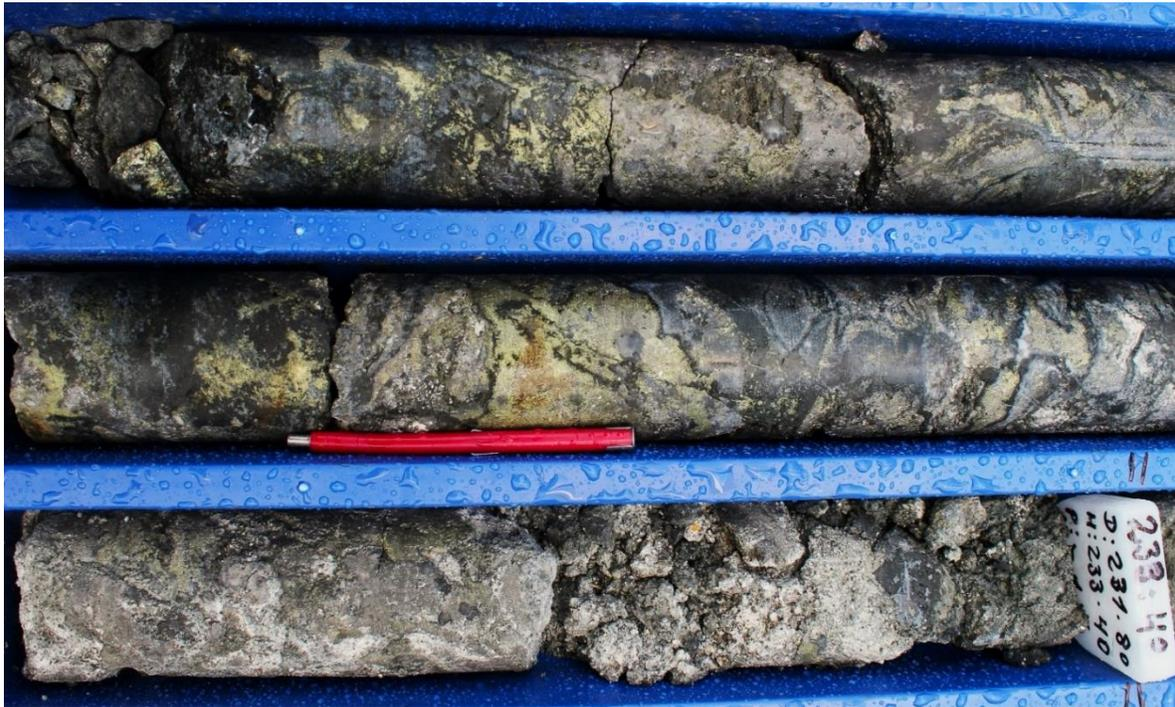
**Figure 6 – High-grade copper mineralisation in drill hole CHT-DDH-041:** Quartz-tourmaline breccia with strongly quartz-sericite-tourmaline altered clasts set in an arsenopyrite-chalcopyrite-pyrite-quartz-tourmaline matrix. From a sample interval (231.63 to 232.34m) that returned 1.2 g/t Au, 105 g/t Ag and 4.6 % Cu. Photograph is of a selected interval and is not necessarily representative of mineralisation hosted throughout the property.
