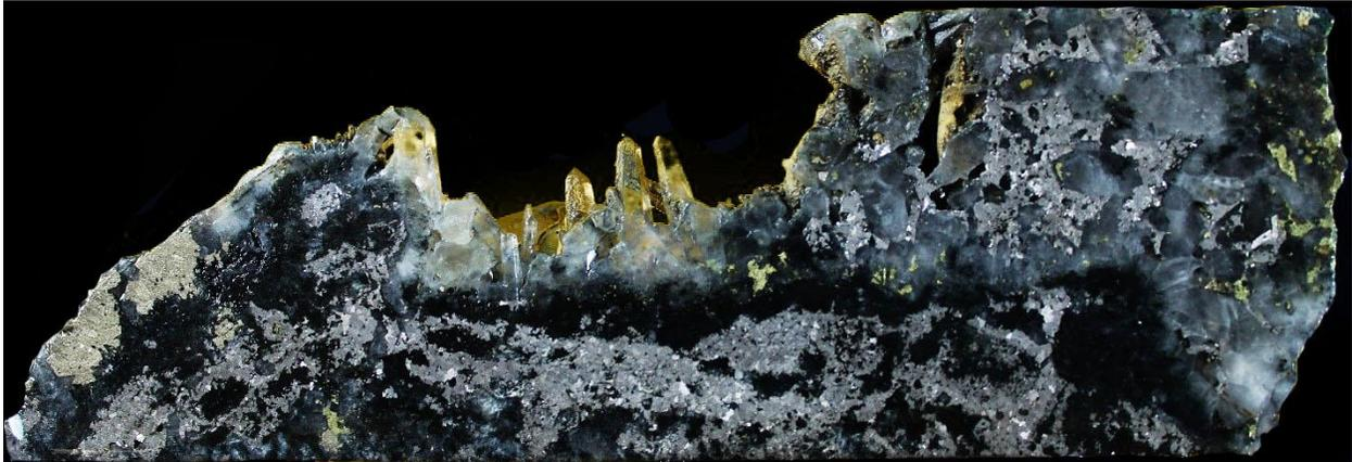
**Figure 8 – Typical high-grade copper-silver mineralisation in drill hole CHT-DDH-041:** Cemented quartz-tourmaline breccia with euhedral quartz and abundant arsenopyrite, chalcopyrite and pyrite. From a sample interval (167.9 to 168.6 m) that returned 2.67 g/t Au, 44 g/t Ag and 1.59 % Cu. Photograph is of a selected interval and is not necessarily representative of mineralisation hosted throughout the property.
