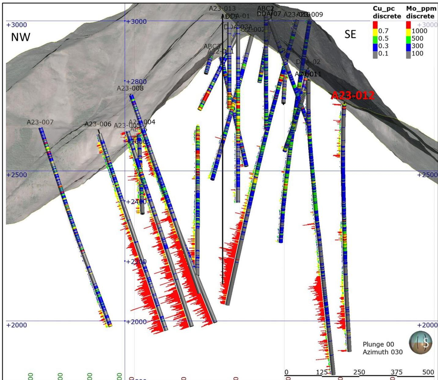
Figure 3: Aurora Project – NW-SE geological section showing DLP and historic drillholes. Downhole values for copper (%) are shown on drillholes with molybdenum (ppm) shown as bar graphs to left of drillholes.
