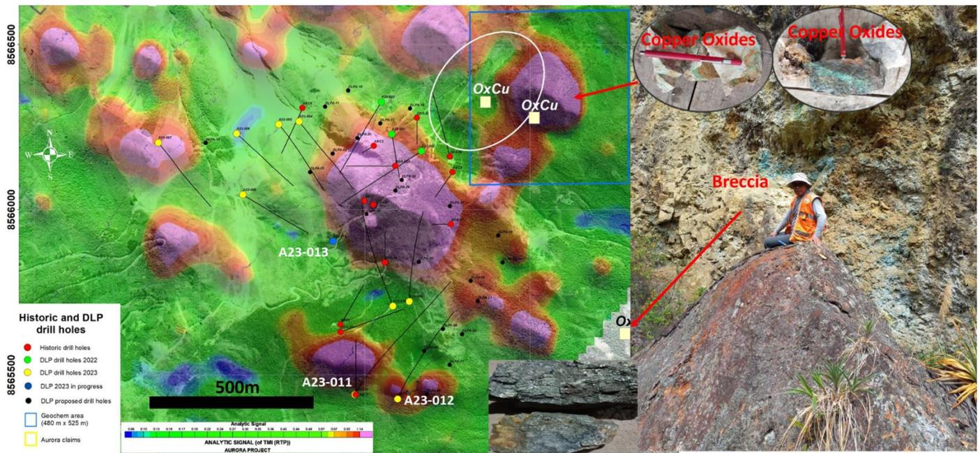
Figure 6: Aurora Project – Magnetic analytic signal data with drillholes shown and new copper oxide showings with planned geochemical grid (blue box).
