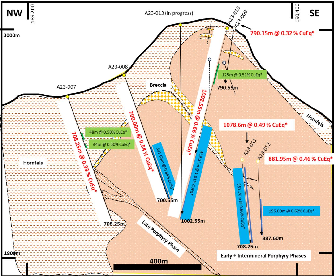
Figure 4: Aurora Project – Simplified NW-SE geological section showing DLP drillholes in yellow dots with summarized mineralized intervals shown alongside drillholes. Green intervals are predominantly copper in CuEq\* calculation and blue intervals are predominantly molybdenum in CuEq\* calculation (Refer to Table 3 for full description).
