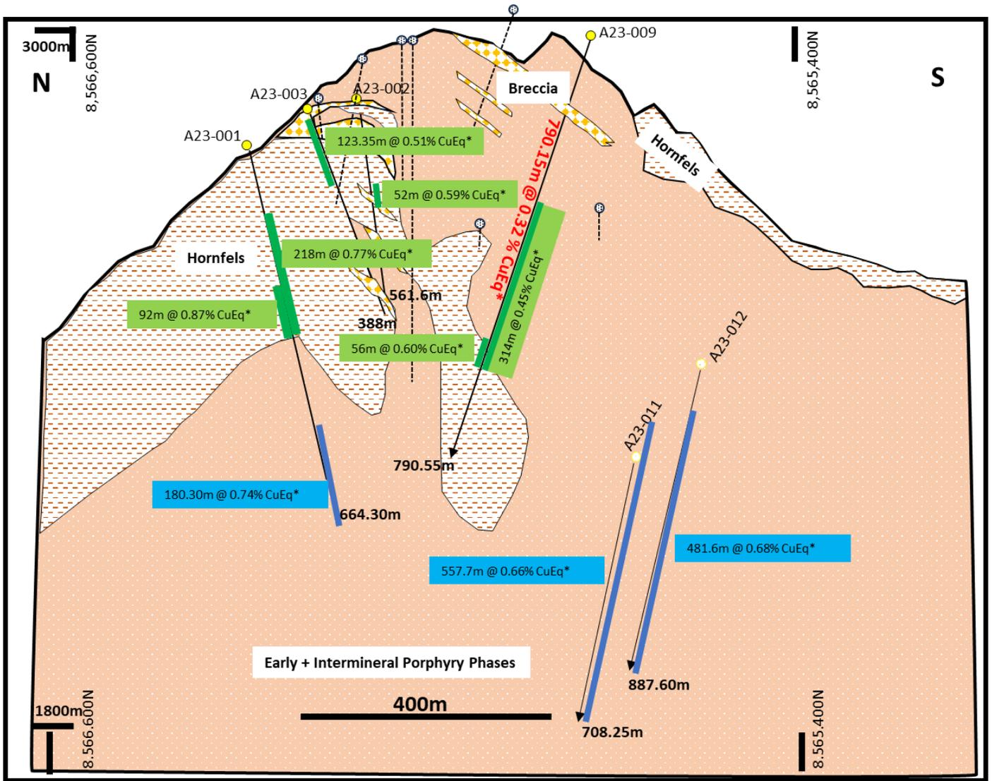
Figure 5: Aurora Project – Simplified N-S geological section showing DLP drillholes in yellow dots with summarized mineralized intervals shown alongside drillholes. Green intervals are predominantly copper in CuEq\* calculation and blue intervals are predominantly molybdenum in CuEq\* calculation (Refer to Table 3 for full description).
