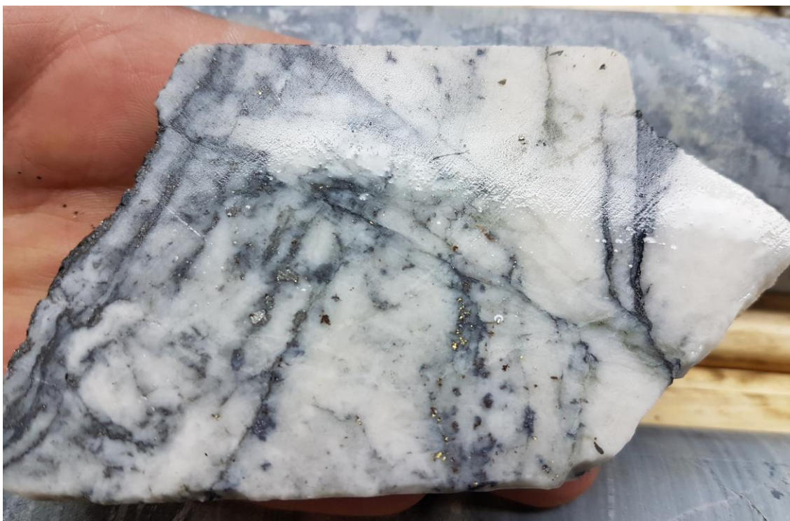
Quartz Vein in GP-21-149 with Visible Gold (238 g/t gold over 0.40 meters core length)
