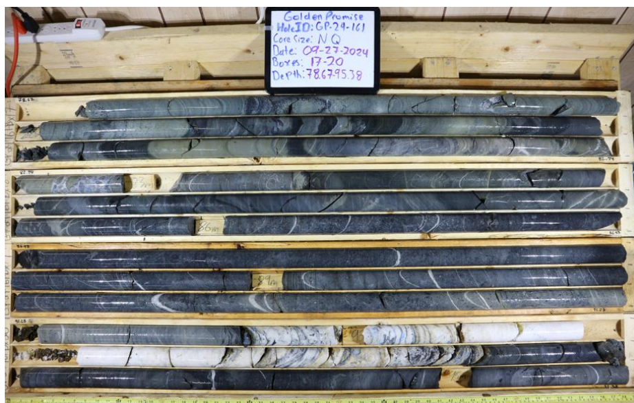
Quartz vein with visible gold in drill hole GP-24-161 (13.16 g/t gold over 1.67 meters core length)
