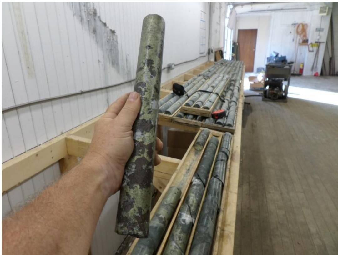
Vein with semi-massive base metal sulfides (sphalerite & chalcopyrite) In Drill Hole Ky-18-14 at Elmtree 12 Vein System (9.04% Zn, 9.19% Cu and 1,158 g/t Ag over 3.00 meters core length)
