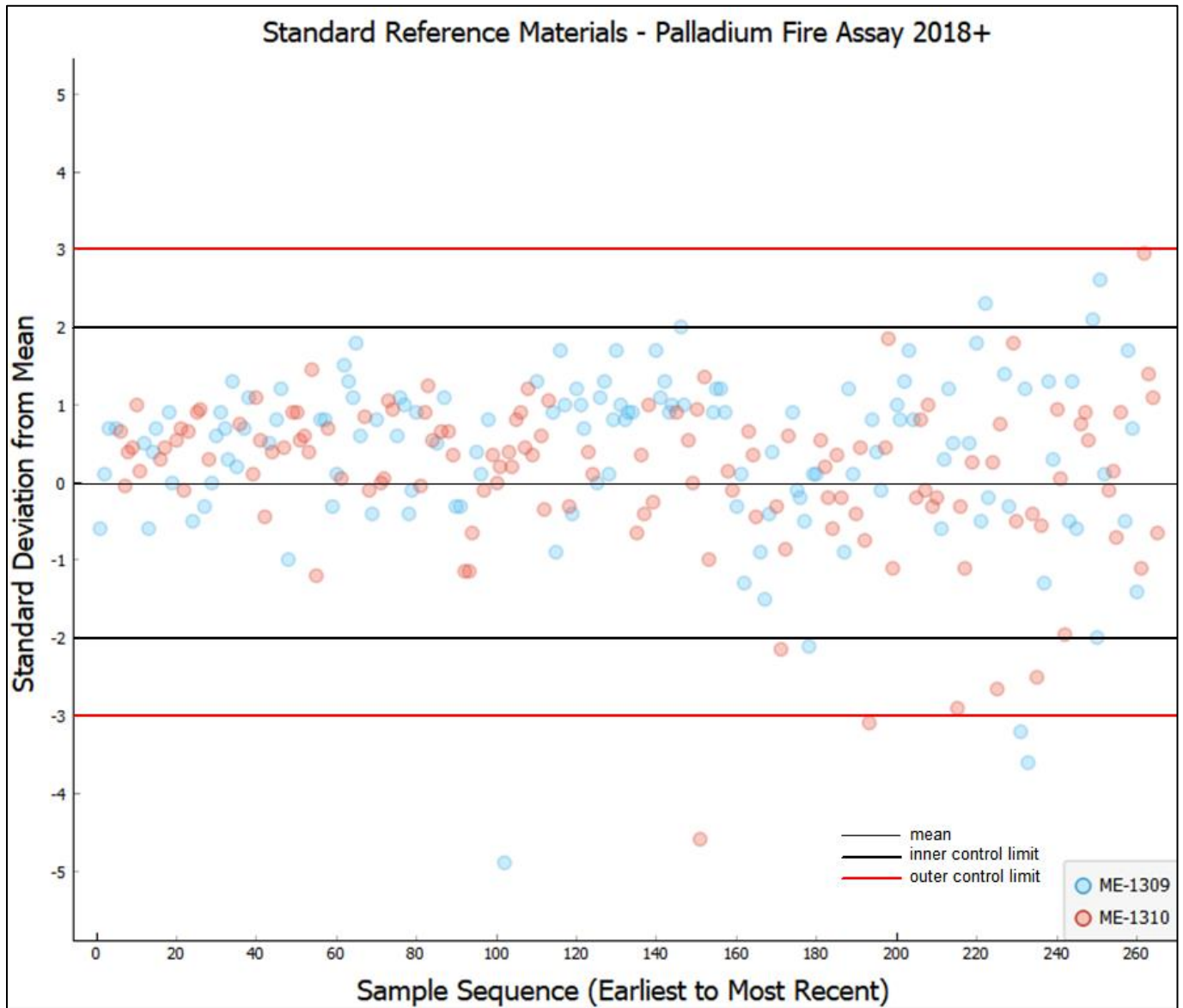
Figure 11-10: Palladium Performance of Standard Reference Materials from 2018 to Present (Source: Giga Metals, 2023)
