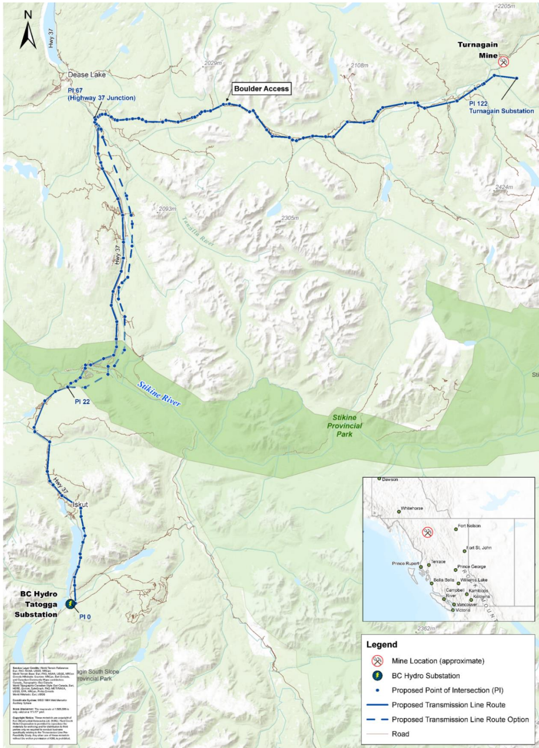
Figure 18-23: Turnagain Mine Preliminary Transmission Line Route (KWL, 2023)
