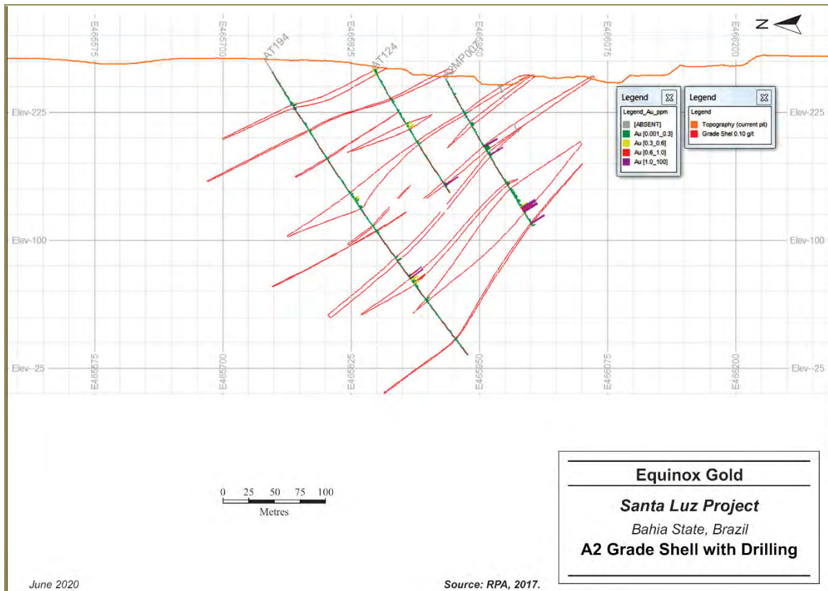
Figure 14-8: Antas 2 Grade Shell with Drilling
