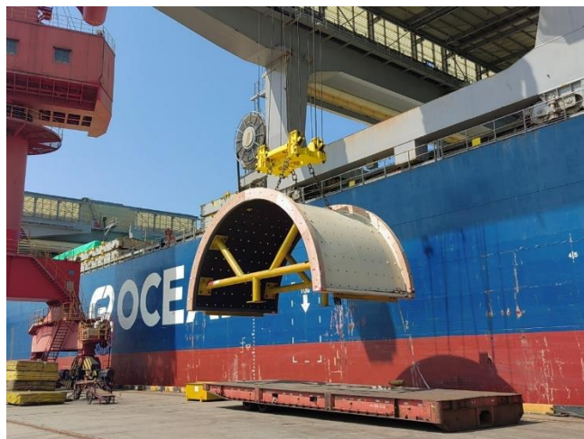
Ball mill shell segment in transit
