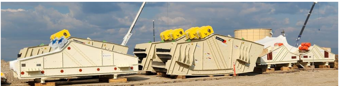
Dry and wet screens
