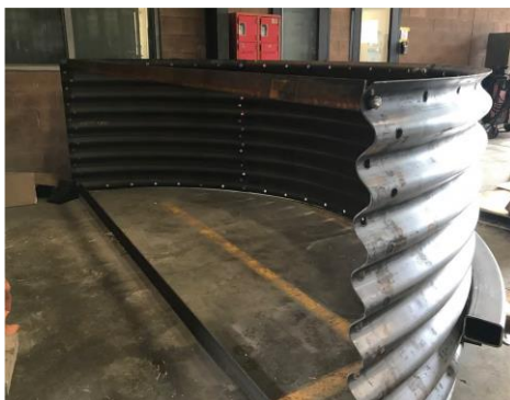
Reclaim tunnel sections
