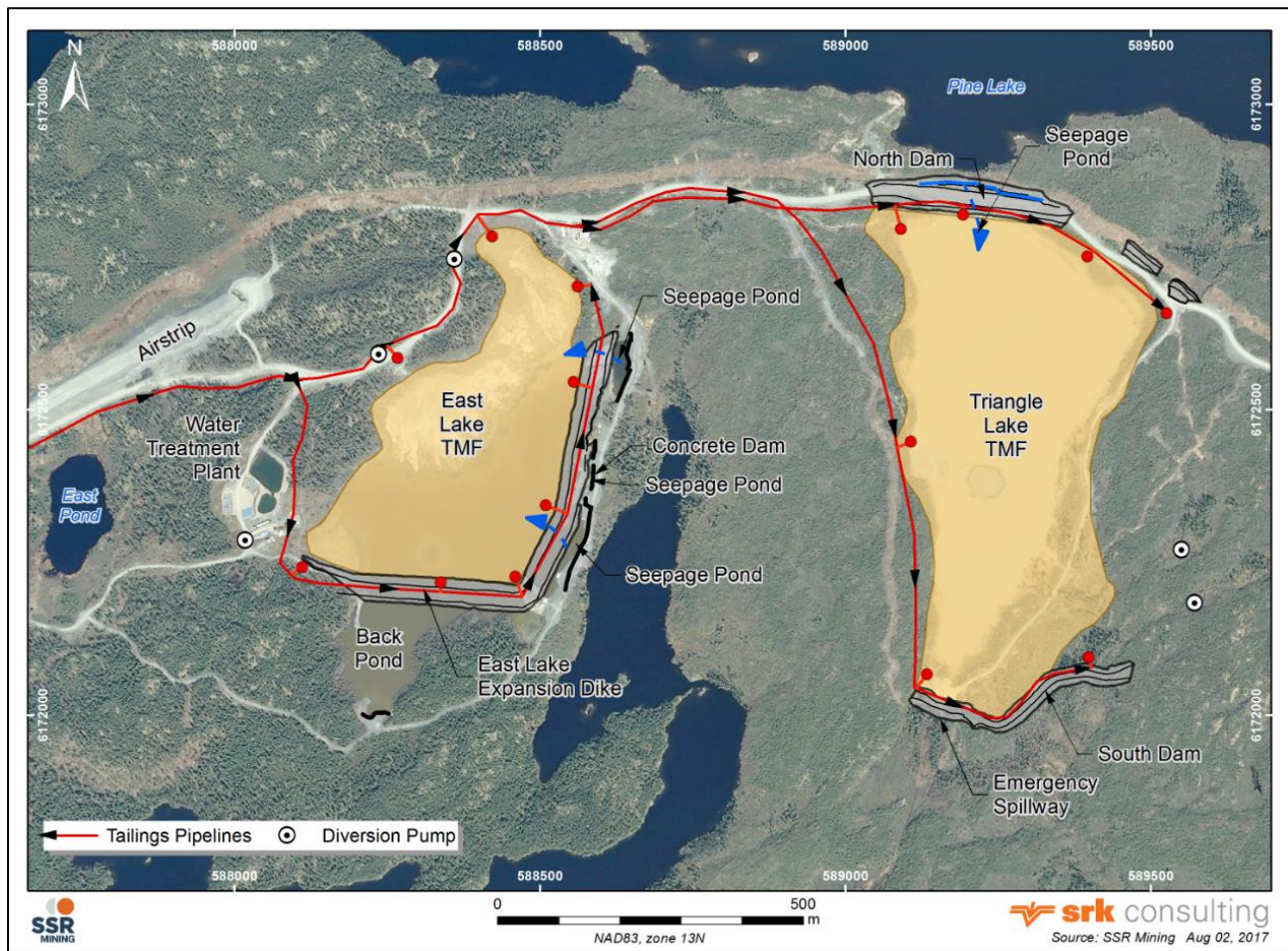
Figure 20: Seabee Gold Operation Tailings Management Facility Infrastructure
