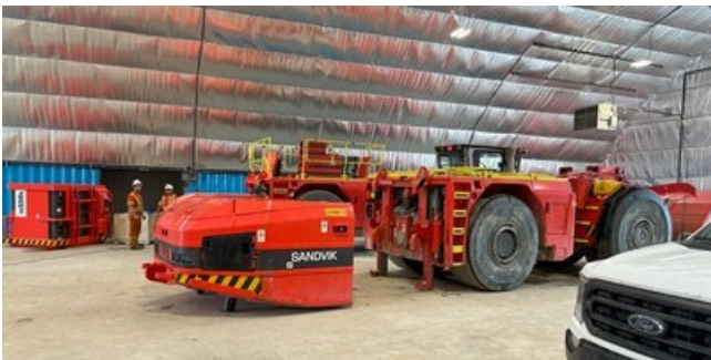
Battery Separation from BEV Scoop (CNW Group/Foran Mining Corporation)
