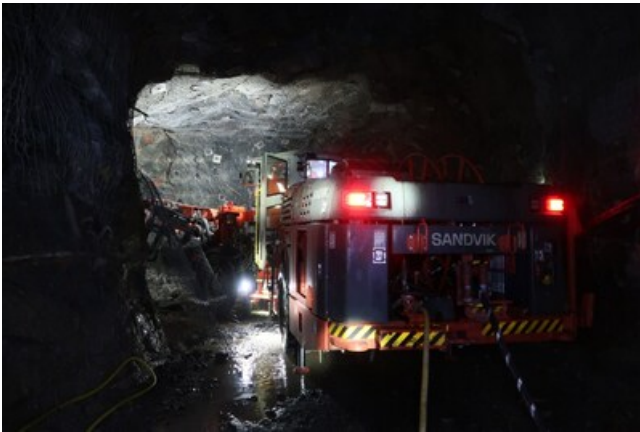
Jumbo Bolting on 60m Level (CNW Group/Foran Mining Corporation)
