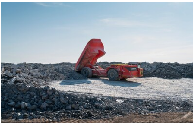
BEV 50T Truck Storing Waste Rock from Underground Development (CNW Group/Foran Mining Corporation)
