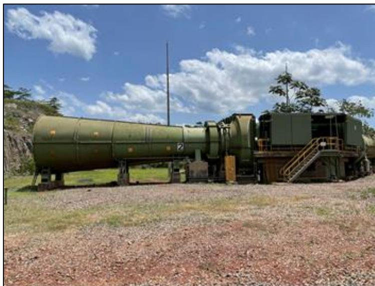
Figure 18-22: Howden Primary Ventilation Fans, Paboase Underground Mine
