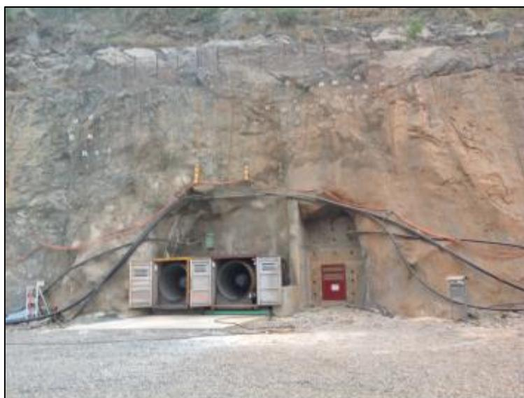
Figure 18-23: Swedvent Primary Ventilation Fans, Akoti Underground Mine
